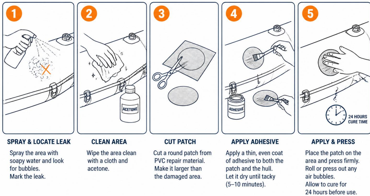
Fig. 7 · Field repair — locate leak, clean, cut round patch, apply adhesive, press & cure.
